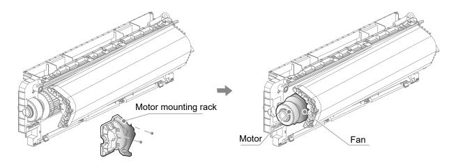
Take the motor and wind wheel out horizontally; loosen the screws fixing the motor and wind wheel, and repair the motor and wind wheel.
