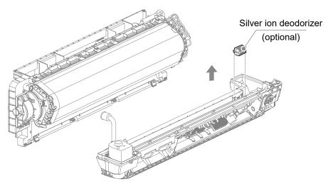
3 Loosen the screw (one), pull the evaporator horizontally a little and hang the evaporator.
