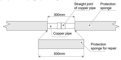
Cut a section of protection sponge longer than the gap, pull open the two ends, insert the protection sponge, and apply glue to the joint.
