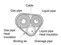
Note: If the drainage pipe is wrapped above the piping, it may cause poor drainage or backflow of water.
