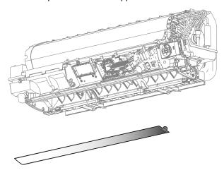
First loosen the screws (three) to remove the display panel, remove the cable terminal on the oscillation motor, then disconnect the left and right louver rod and the left and right swing motor rod, and take the swing motor and repair it.
