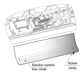
Connect the strong current wires (power cable, alarm signal output wire, and strong current sterilization wire) and weak current wires (communication line, function expansion board connection wire, remote switch connection wire) to the electric control box through the bottom of the electric control box, and the strong and weak current inlets.
