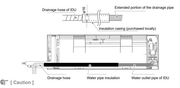
Indoor parts of the drainage pipe shall be insulated to prevent condensation, and protective sleeves should be thicker than 10mm.
